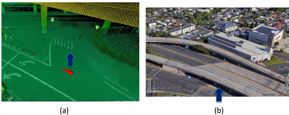
Figure 27. Crosswalk (a) detected by LiDAR, and (b) obstructed from satellite imagery
