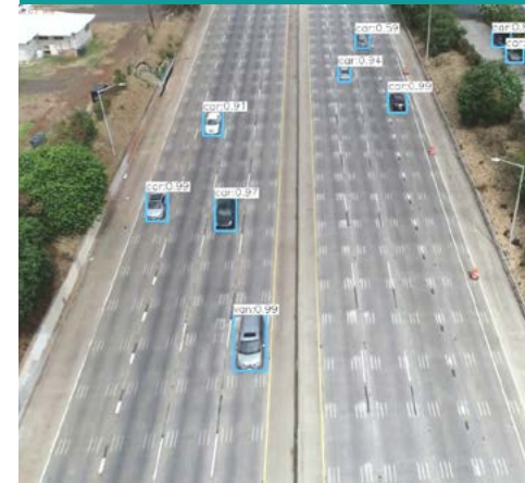
Above: Screenshot of the output video. The markers show positions of the detected vehicles.
