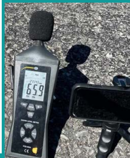
Sound Meters field setup used for data collection.
