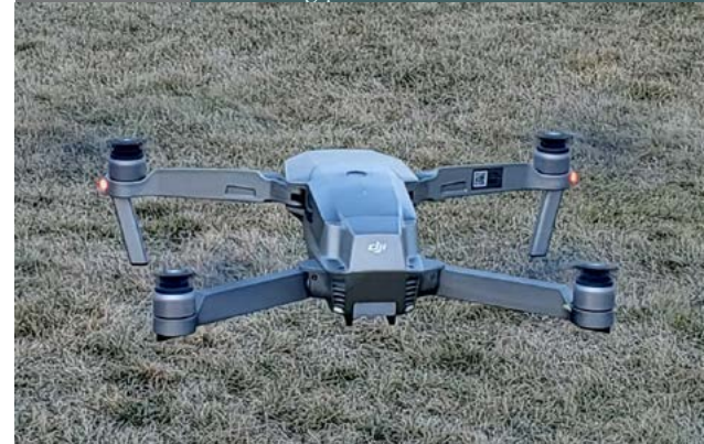
The DJI Mavic Pro Platinum quadcopter drone used for collecting video to analyze for pedestrian data at 3 schools in Moscow, Idaho.
