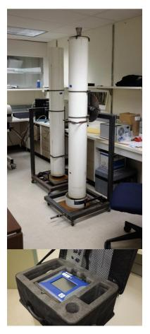
Figure 2-1. The dustfall column and the aerosol sensor used to record data for the UAFDUST application.
