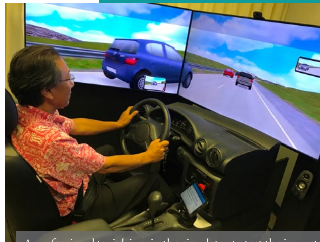
A professional taxi driver in the simulator to test the impact of text distractions while driving in set conditions.
